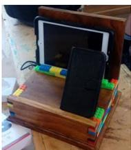
shows a charging station built by Scott Syder in his Year 12 Technology class. Scott printed the Lego bricks on the 3D printer to make the sides of his stand.
